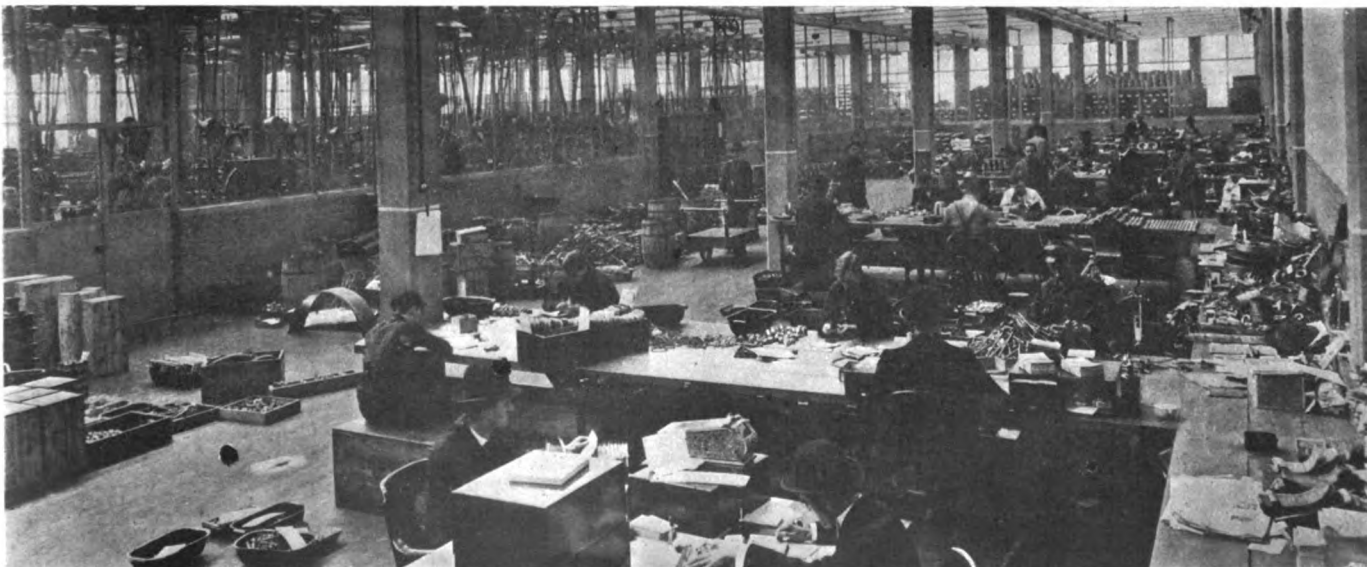
In the Inspection Room Each Workman Has a Desk and Is Seated at the Careful Work of Checking Up Parts Dimensions.
